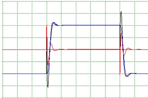
Figure 1. Square wave response of a 4<sup>th</sup> order Linkwitz/Riley crossover.
